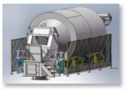
Easy access for daily clean up. – Removable inlet ring provides access for removal and insertion of paddles and discharge blades
